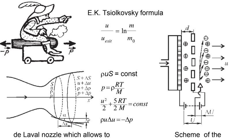
accelerate the gas over sound velocity
