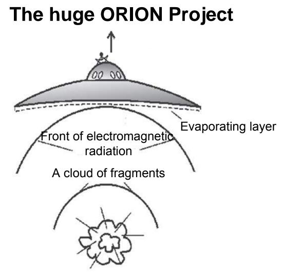
The step-by-step acceleration of the vehicle is provided with the explosions of atom bombs
